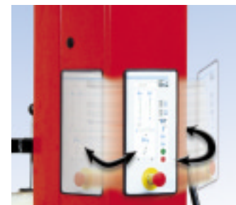
The control panel can be positioned on the right, left or rear of the tower.
