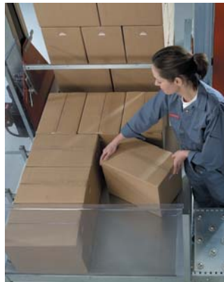
On the stripper plate, the operator forms the desired pattern.
